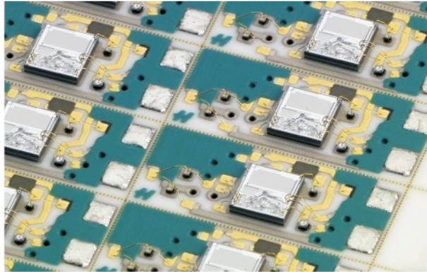
**HYBRID SA** IS ABLE TO BOND CHIPS OF DIFFERENT SIZE AND THICKNESS ON DIFFERENT TYPES OF SUBSTRATES. POSITIONING ACCURACY AND OTHER PRODUCT SPECIFICATIONS ARE DETERMINED IN COLLABORATION WITH THE CLIENT.
